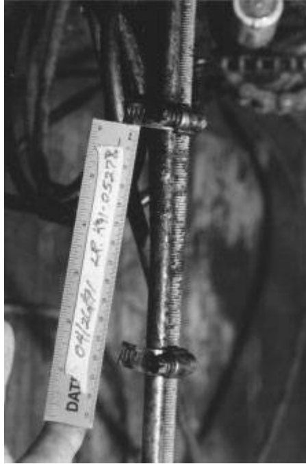
Figure 8.84 The throttle cable, routed through the floor of deck, with blood-stains and hair on its surface.
